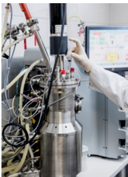
Bioreactor in which biodegradation on a semi-technical scale was carried out and process parameters were monitored
