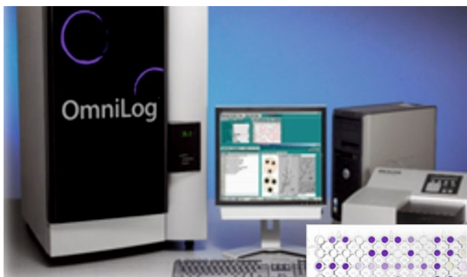
BIOLOG® system for identification of bacterial multiple resistance and MIC (Minimum Inhibitory Concentration) determination for several tens of antibiotics from different chemical groups
